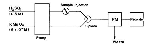
Fig. 1. FI manifold for the chemiluminescent determination of cefadroxil monohydrate: P, peristaltic pump; S, sample port; T, perspex T-piece; L, luminometer; W, waste.
