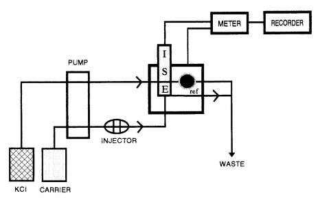
Fig. 1. FIA manifold and experimental set-up used in the study. Carrier stream consisted of 0.001 mM paraquat dichloride in Trizma base buffer (pH 5.5); reference stream was 10 mM KCl solution.
