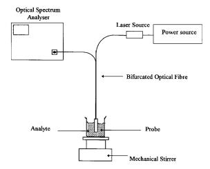
Fig. 1. Schematic diagram of the mercury(II) fibre-optic sensor instrumentation.
