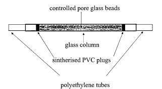
Fig. 1. Schematic design of the enzyme reactor.
