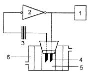
Fig. 1. Schematic diagram of the SPQC system. (1) Frequency counter; (2) IC-TTL oscillator; (3) quartz crystal; (4) conductivity electrodes; (5) detection cell; (6) thermostatic waterjacket.
