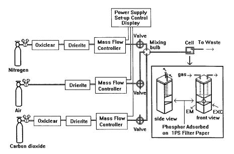
Fig. 1. Experimental system for continuous gas-flow for oxygen sensing.
