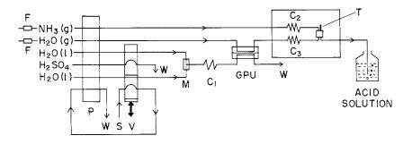
Fig. 1. Schematic diagram of the dual-phase gas-permeation flow-injection manifold for the thermometric determination of carbonate. F, air filter; T, thermistor flow-through detector; W, waste; P, peristaltic pump; V, sampling valve; M, mixing tee; GPU, gas-permeation unit;  $C_1$ , reaction tube;  $C_2$  and  $C_3$ , temperature equilibration coils; S, Na<sub>2</sub>CO<sub>3</sub> sample; g, gas; and l, liquid.
