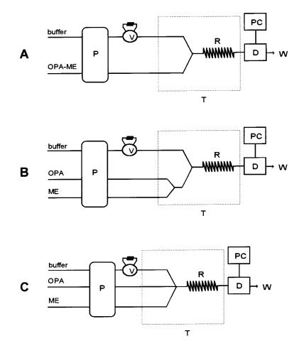
Fig. 1. FI systems used for the determination of amines using the OPA–ME reaction. A, manifold selected; P, peristaltic pump (total flow-rate 0.9 ml min<sup>-1</sup>); V, injection valve (sample-loop 360  $\mu$ l); R, reactor coil (1.5 m long and 0.8 mm i.d.); T, thermostat at 25°C; D, fluorimeter (336/455 nm (excitation/emission)); PC, personal computer; W, waste.
