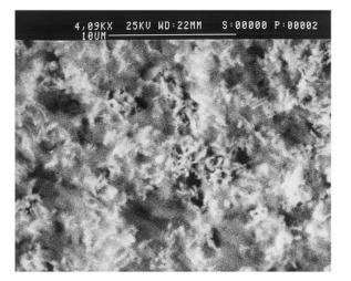
Fig. 9. Scanning electron micrograph of the alloy substrate covered with treated polymer layer (according to method V).
