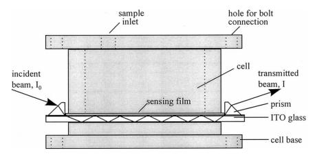
Fig. 2. Experimental arrangement for ATR spectrometry.
