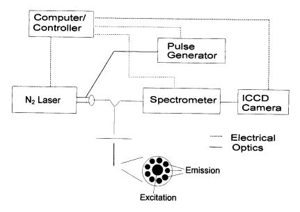
Fig. 1. Schematic representation of the time-resolved, laser-induced fluorescence (LIF) system as deployed in situ.
