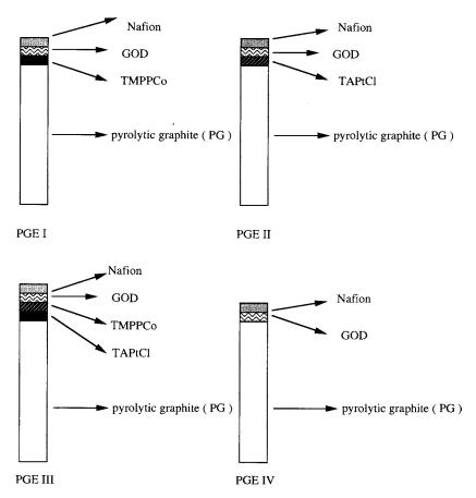
Fig. 1. Schematic graph of the composition of the four kinds of glucose electrodes.
