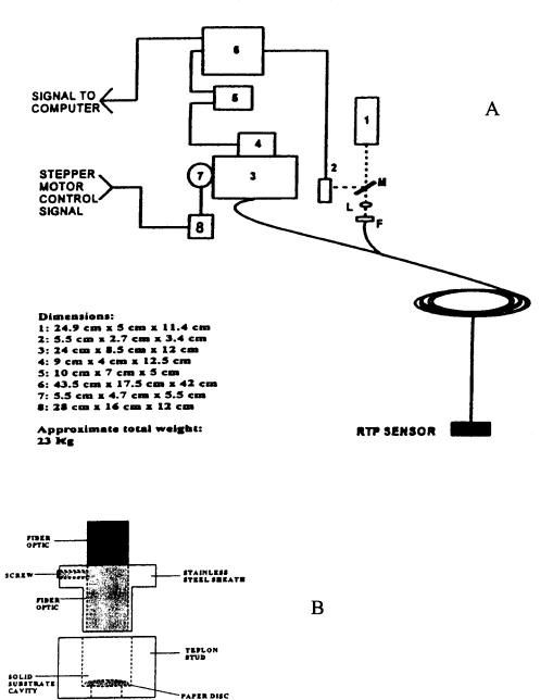
Fig. 6. (A) Block diagram of the laser system employed with the laser-induced RTP sensor. 1 = Nitrogen laser; 2 = photodiode trigger; 3 = monochromator; 4 = PMT; 5 = preamplifier; 6 = boxcar; 7 = motor; 8 = motor control; L = lens; M = reflecting surface; F = fiber optic mount. (B) Cross-section of the RTP sensor.
