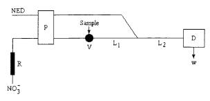
Fig. 1. Flow injection assembly for metoclopramide hydrochloride determination. D, spectrophotometer; L, reactor lengths; P, peristaltic pump; R, solid-phase reactor; V, injection valve.
