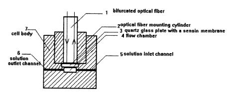
Fig. 1. Schematic diagram of the flow cell arrangement.
