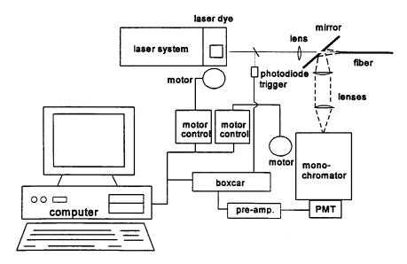
Fig. 5. Schematic diagram of the laser synchronous fluorescence fiberoptic sensor.
