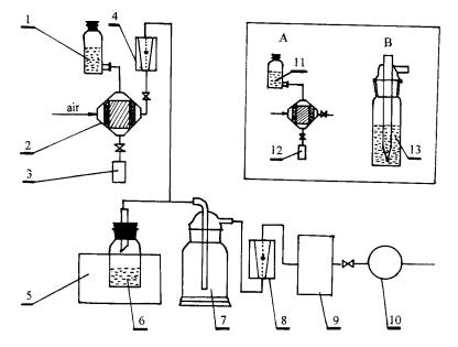
Fig. 6. The device for the comparison between chromatomembrane cell and impinger: (1) 2.0 M NaOH; (2) chromatomembrane cell 1; (3) collector for waste solution; (4) rotameter 1 for free-fluorine air; (5) thermostatical water bath; (6) HF solution (15%) (7) mix chamber; (8) rotameter 2 for sample air; (9) absorbing device (A or B); (10) pump, (11) 0.10 M NaOH, (12) collector for sample solutions, (13) 0.10 M NaOH.
