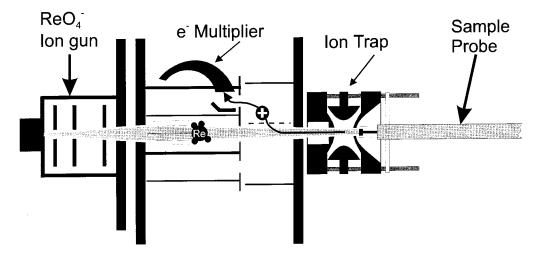
Fig. 1. Schematic diagram of the ion trap SIMS instrument.
