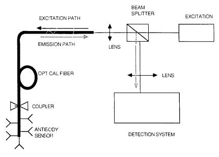
Fig. 8. The anibody-based biosensor for benzo[a]pyrene.
