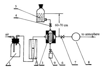
Fig. 2. Scheme of experimental device for absorption of fluorine in air: (1) buffer bottle; (2) rotameter; (3) chromatomembrane cell; (4) and (6) regulating valve for absorbing solution; (5) 0.10 M NaOH; (7) air regulating valve; (8) pump; (9) samples solution collector.
