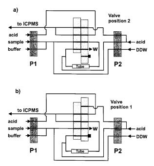
Fig. 1. FI manifold for on-line trace metal separation and preconcentration. P1, pump 1; P2, pump 2; W, waste. (a) Sample loading and wash; (b) elution.
