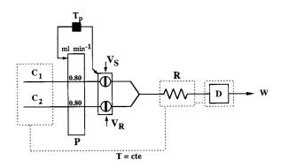
Fig. 1. Flow system. P, peristaltic pump;  $C_1$ ,  $C_2$ : 0.2 M phosphate buffer, pH 6.5, 0.80 ml min<sup>-1</sup>;  $V_S$ : sample injector, 115  $\mu$ l;  $V_R$ : reagent injector, 198  $\mu$ l; R: coiled PTFE tube, 300 cm long, 0.5 mm i.d.;  $T_p$ : timer; D: detector; W: waste; working temperature is kept constant by means of a water-circulation thermostatic bath.
