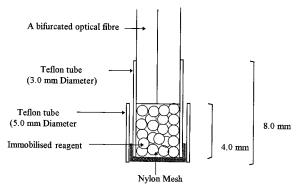
Fig. 2. The design of the mercury(II) probe.
