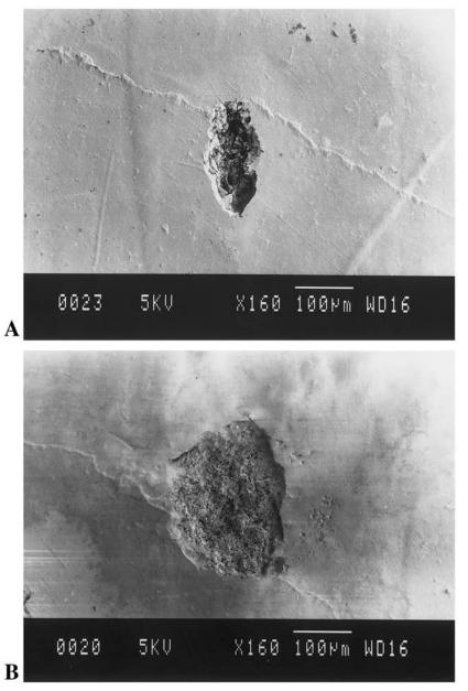
Fig. 3. Scanning electron micrographs of  $10000V-2TiO_2-SiO_2$  sample, showning the craters produced after two cummulative laser shots. (A) Sample placed at the focusing lens focal position. (B) Sample placed 2 mm below the focusing lens focal position.
