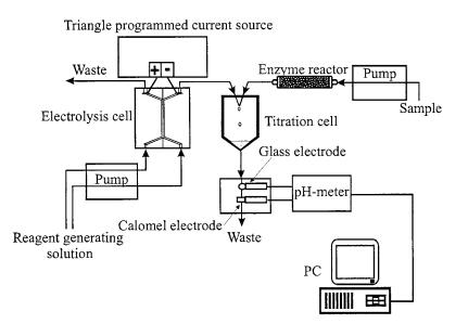
Fig. 2. The schematic design of the triangle programmed coulometric flow titration system.
