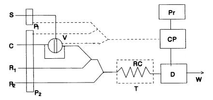
Fig. 1. Schematic diagram of the flow-injection system used for the determination of nitrite. S, sample; C, carrier;  $R_1$ , potassium bromate in phosphoric acid solution;  $R_2$ , naphthol green B;  $P_1$ ,  $P_2$ , peristaltic pumps; V, injection rotary valve; RC, reaction coil; T, thermostatic water bath; D, detector; CP, computer controlling and data processing system; Pr, printer.
