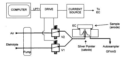
Fig. 1. Flow diagram of the proposed system. Three-way solenoid valves (V1 and V2); electrolytic cell (EC); exit to printer (LPT1); polyethylene tubes (—) and electric contacts (—).
