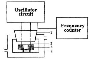
Fig. 1. Schematic depiction of the system for detection of *E. coli.* (1) Rubber plug. (2) Leading wire. (3) Well-type detection cell. (4) Thermostatic jacket.
