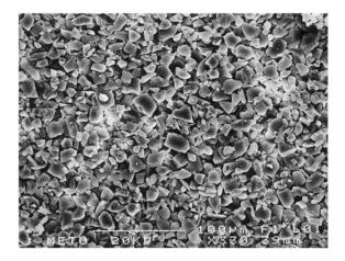
Fig. 4. SEM photograph ( $\times$  330) of commercial silica gel plate surface treated with 0.5 M CdCl<sub>2</sub> and exposed to 0.870 ppm H<sub>2</sub>S for 60 min.
