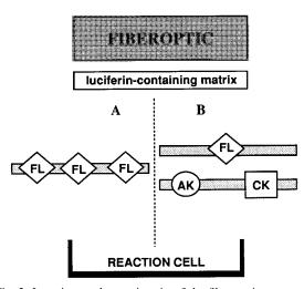
Fig. 2. Location at the sensing tip of the fibre-optic sensor of the luciferin-containing matrix when associated with the firefly luciferase membrane alone (A) and with the compartmentalised adenylate kinase-creatine kinase-firefly luciferase system (B).
