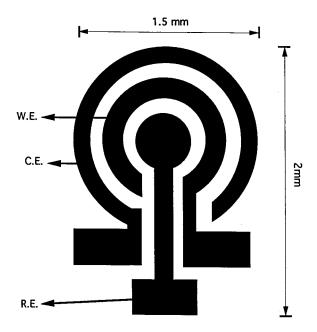
Fig. 1. Schematic of a designed microsensor system with working electrode (WE), reference electrode (RE) and counter electrode (CE).
