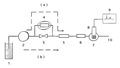
Fig. 1. Schematic diagram of the system. 1, buffer tank; 2, peristaltic pump; 3, injection port; 4, AlP-reactor thermostated; 5, Np-reactor; 6, XO-reactor; 7, flow cell; 8, screen-printed electrode; 9, recorder; 10, waste. (a) the sample flows through the AlP-reactor and the current obtained is proportional to the sum of IMP, HxR, Hx and UA. (b) the sample flows through the valve and the current obtained is proportional to the sum of HxR, Hx and UA.
