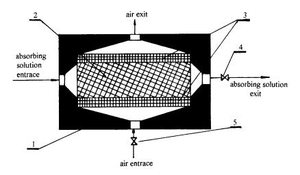
Fig. 1. Chromatomembrane cell: (1) case of the cell; (2) mass-exchange layer; (3) microporous membrane; (4) regulatory valve for absorbing solution; (5) air regulatory valve.
