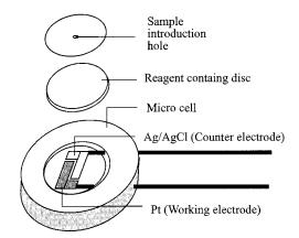
Fig. 1. Amperometric microcell for enzyme activity measurements. The microfabricated electrochemical cell (on flexible polyimide Kapton<sup>®</sup> with traces, and bonding pads) is embedded in a poly(methyl methacrylate) plastic body. The small volume space, (6 mm diameter and 800 μm thickness) holds the reagent-containing porous membrane disc and/or liquid reagent film. To avoid solvent evaporation a plastic cover slide was used during measurements.
