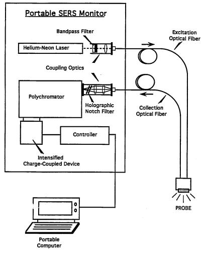
Fig. 7. The Portable SERS fiberoptic sensor.
