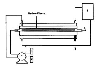
Fig. 2. Schematic representation of the equipment with the hollow fiber module used in permeation experience of metals with LIX 864. (1: donor solution, 2: stripping solution, 3: peristaltic pump, 4: outlet stripping (sample), 5: outlet donor solution (sample), 6: thermostatic bath).
