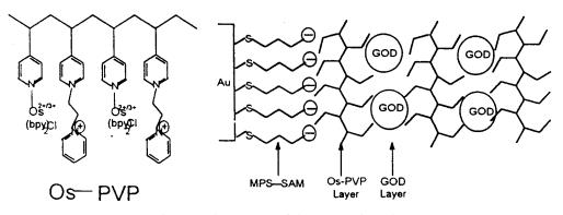
Scheme 1. The structure of the enzyme electrode.
