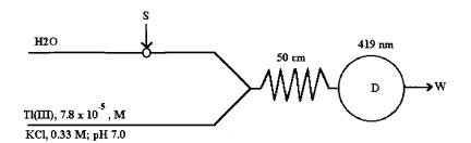
Fig. 1. Schematic diagram of the flow injection system.
