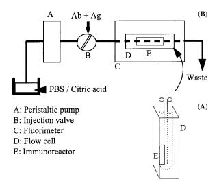
Fig. 1. (A) Flow-cell, (B) flow injection system.
