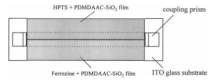
Fig. 1. Schematic pattern of the Ferrozine and HPTS immobilized PDMDAAC-SiO<sub>2</sub> film for dual-analyte (Fe<sup>2+</sup> and pH) sensing. The dashed lines indicate the path of the interrogating light that undergoes multiple internal total reflection within the glass substrate as a result of prism coupling.
