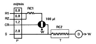
Fig. 1. Manifold optimized for the determination of nicotine. R1, potassium cyanide solution; R2, chloramine-T solution; CR, chromogenic reagent; S, sample solution; RC1, reaction coil (50 cm  $\times$  0.8 mm i.d.); RC2, reaction coil (300 cm  $\times$  0.8 mm i.d.); P, peristaltic pump; T, thermostatic bath; D, photometric detector; W, waste.
