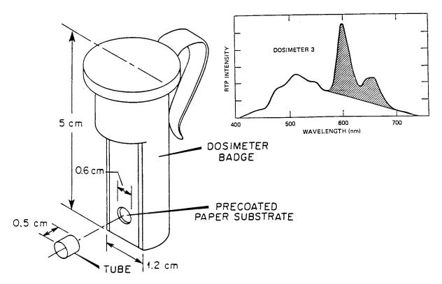
Fig. 4. The vapor dosimeter for polyaromatic compounds. The insert (upper right curve) shows the RTP spectrum of pyrene vapor (shaded area) detected at an industrial site.
