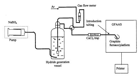
Fig. 1. Schematic of the hydride generation, introduction, deposition and atomization.
